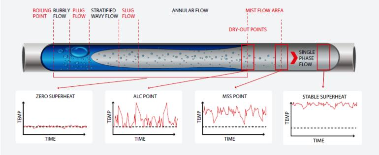
Utilization of the evaporator surface is maximized while ensuring that no liquid exits the evaporator – safeguarding the compressor and delivering significant energy savings and optimal food safety.
